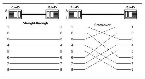
The cable connection of RJ-45 connector conforms to the 568B standard (1-orange white, 2-orange, 3-green white, 4-blue, 5-blue white, 6-green, 7-brown white, 8-brown).
